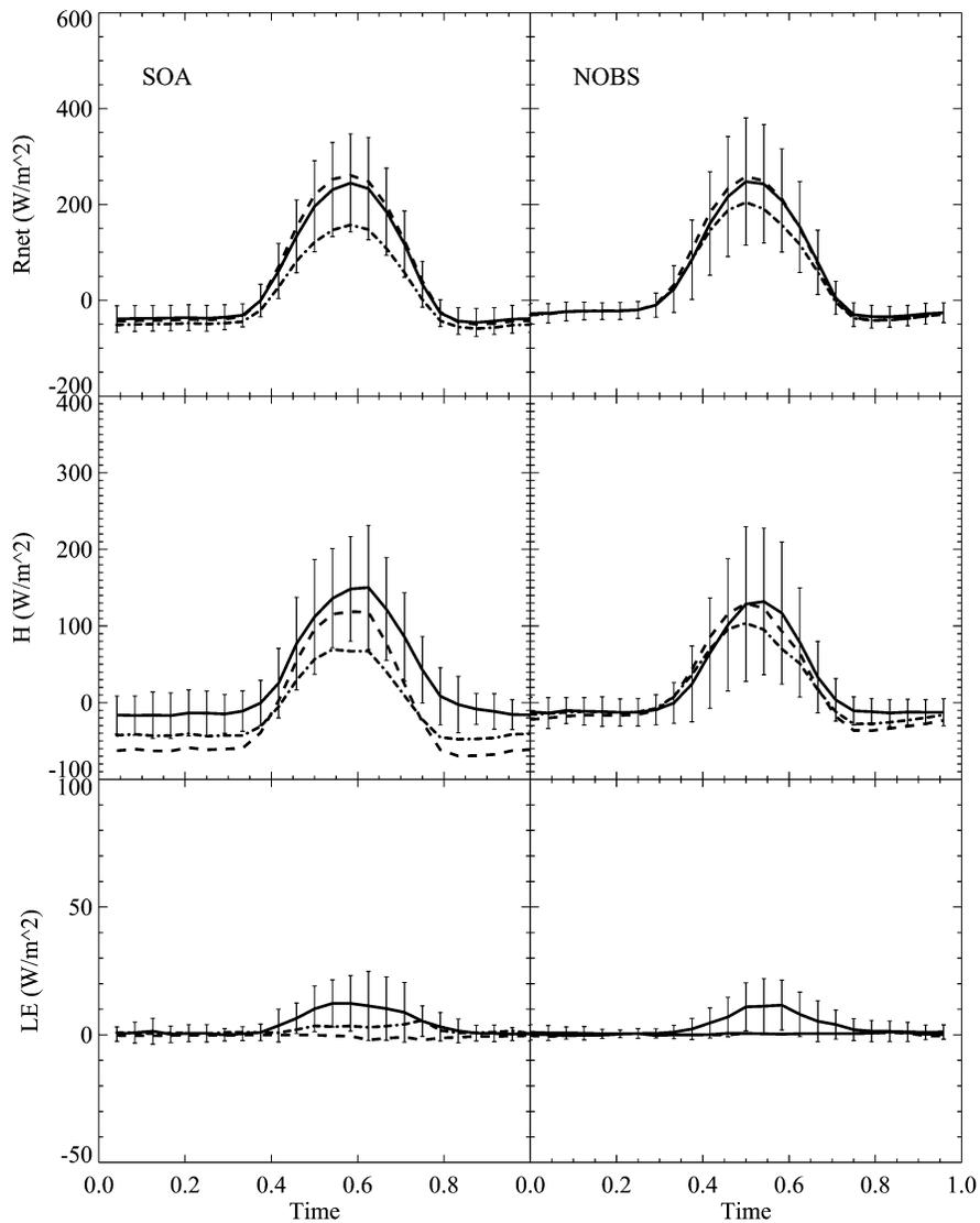
**Figure 5:** comparison of the measured (solid lines) with standard deviation and modeled (VIC: dashed and dotted lines and VIC-CCS: dashed lines) climatological winter diurnal curves of net radiation ( $R_{net}$ ), sensible heat fluxes ( $H$ ) and latent heat fluxes ( $LE$ ) in the old aspen stand in the southern study site (SOA, for 1994) and the old black spruce forest stand in the northern study site (NOBS for 1995) of the boreal forest in central Canada. 0.5 is the local solar noon.
