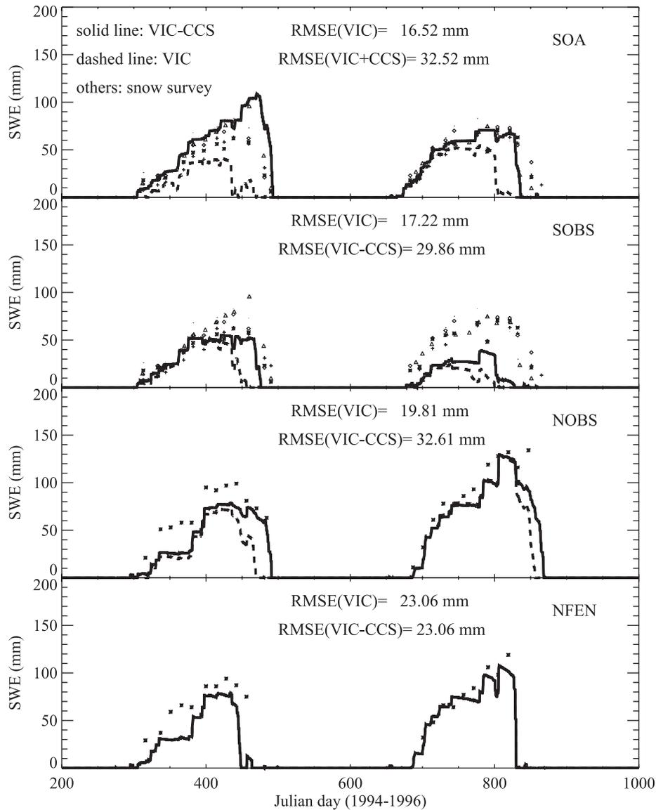
**Figure 7:** comparison of the modeled SWE and the snow surveys in the SOA, SOBS, NOBS and NFEN sites from 1994 to 1996.
