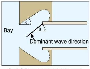
Figure 12. Equilibrium inner-bank erosion showing dominant wave angle and shoreline orientation angle,  $\beta$
