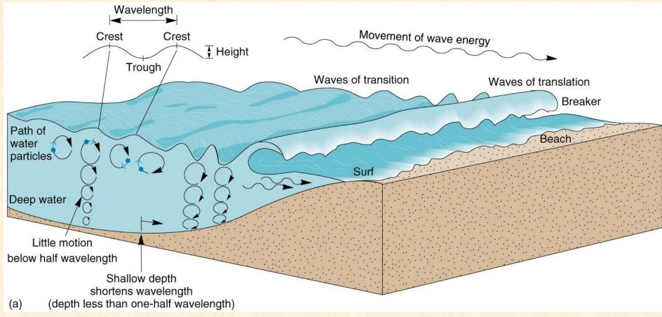
**Shallow Water Processes**: shoaling, refraction, diffraction, reflection, breaking, wave(wind) setup/setdown
