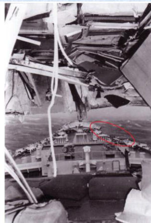
(b) View from inside a cabin through the torn superstructure of the Michelangelo after it was hit by a rogue wave. Note the missing section of bow on the right side of the ship (red oval).
