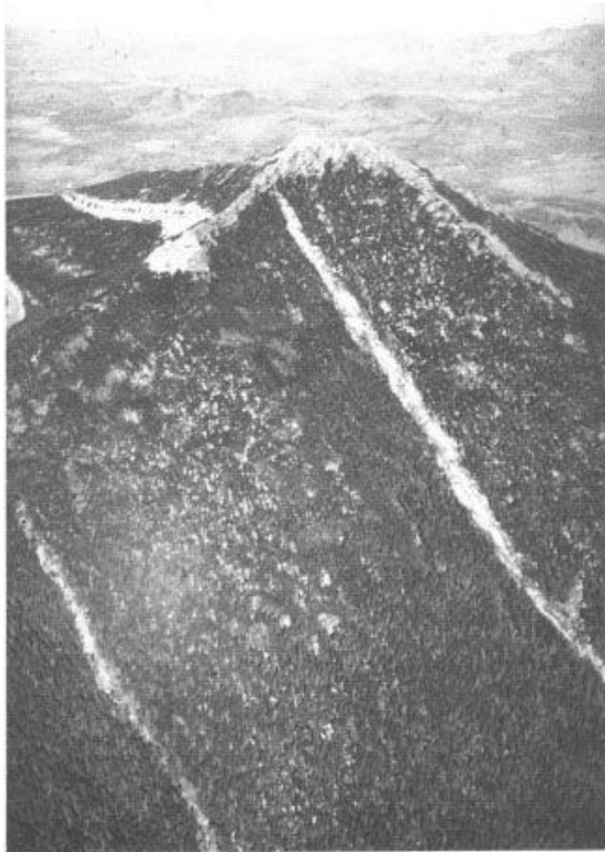
Figure 14.1. In this aerial view of Whiteface Mountain, you can see the long, narrow, light-colored scar left by a landslide. Rock slides like this one can happen on steep, smooth rock slopes. A very heavy, once-in-a-lifetime downpour soaks the carpet of vegetation so thoroughly that it no longer sticks to the rock. Then the forest mat crashes down the mountain.
