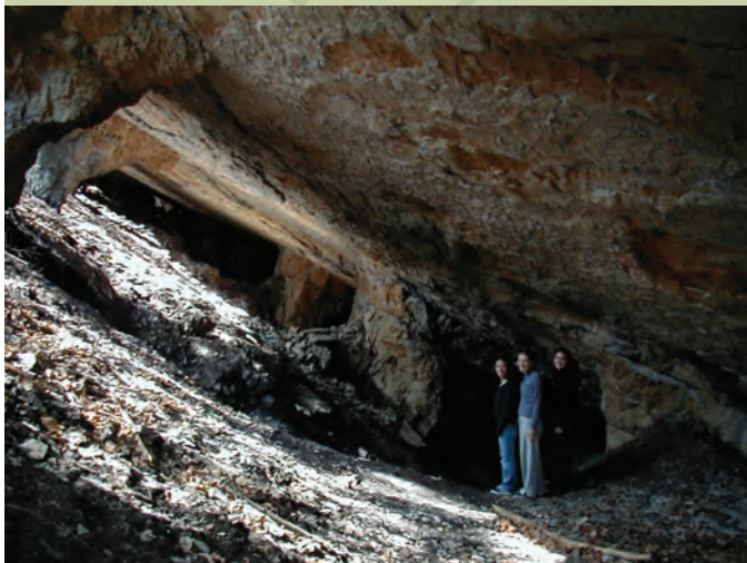
► Figure NY-NJ.26 Rosendale cement was mined using the room and pillar method wherein the roof of the mine is supported by pillars of unmined rock. Abandoned mines such as the one pictured here are common in the Rosendale-Tillson area of New York. Several mines are now used as underground storage facilities for corporate document archives and for mushroom farms.
