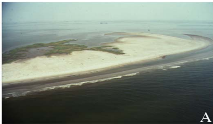
Figure 5. Photographs taken 7 weeks apart of the east end of Timbalier Island illustrating the severe erosion that occurred along the margin of Little Pass Timbalier during Hurricane Andrew: A) Before - taken July 9, 1992, and B) After - taken August 30, 1992.
